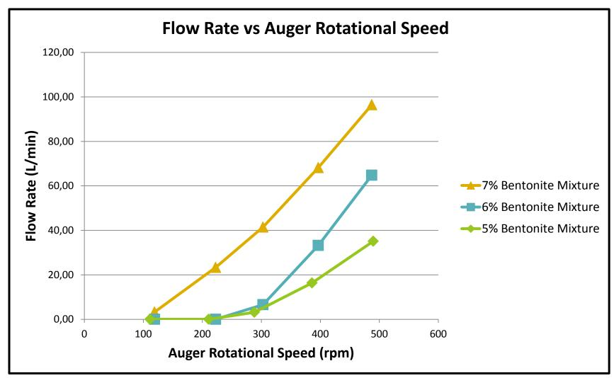
Flow rates produced for varying auger rotational speeds at 22.5% submergence with three concentrations of simulated waste.
