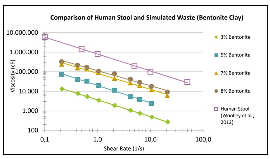
Viscosity vs. shear rate for human stool (Woolley et al., 2012) and simulated waste (varying concentrations of bentonite clay)
