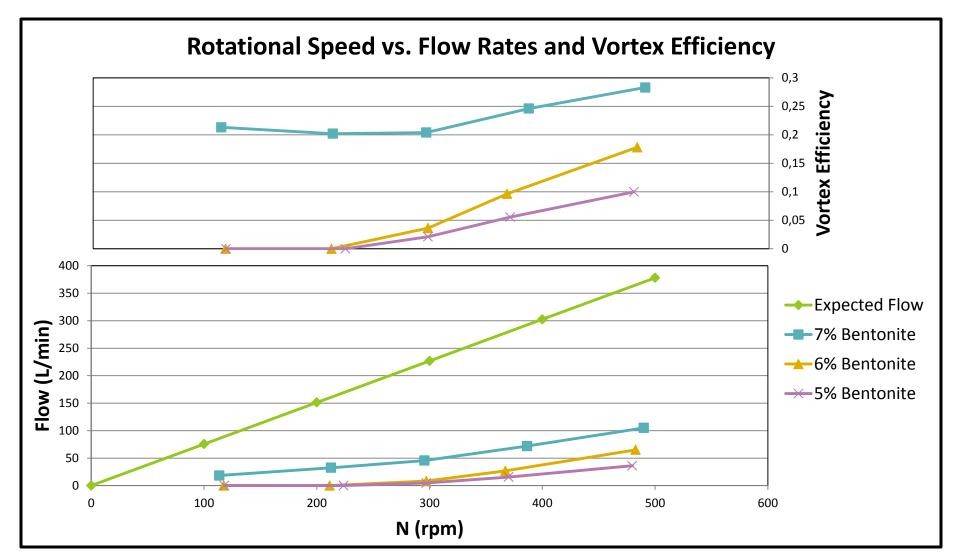
Flow rates and corresponding vortex efficiencies produced for varying auger rotational speeds at 32.5% submergence with three concentrations of simulated waste.
