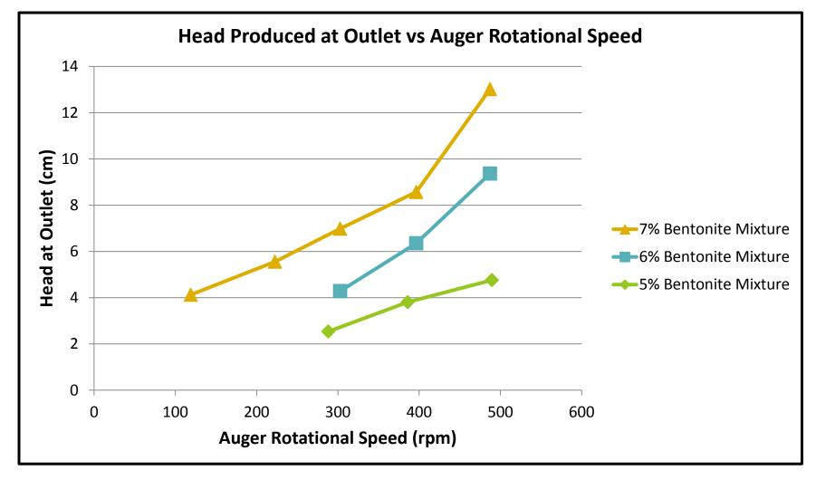
Head produced at outlet for varying auger rotational speeds at 22.5% submergence with three concentrations of simulated waste.
