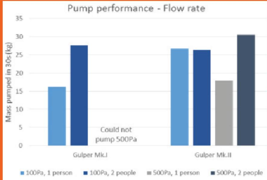
Figure 2 – Results of pump performance testing
