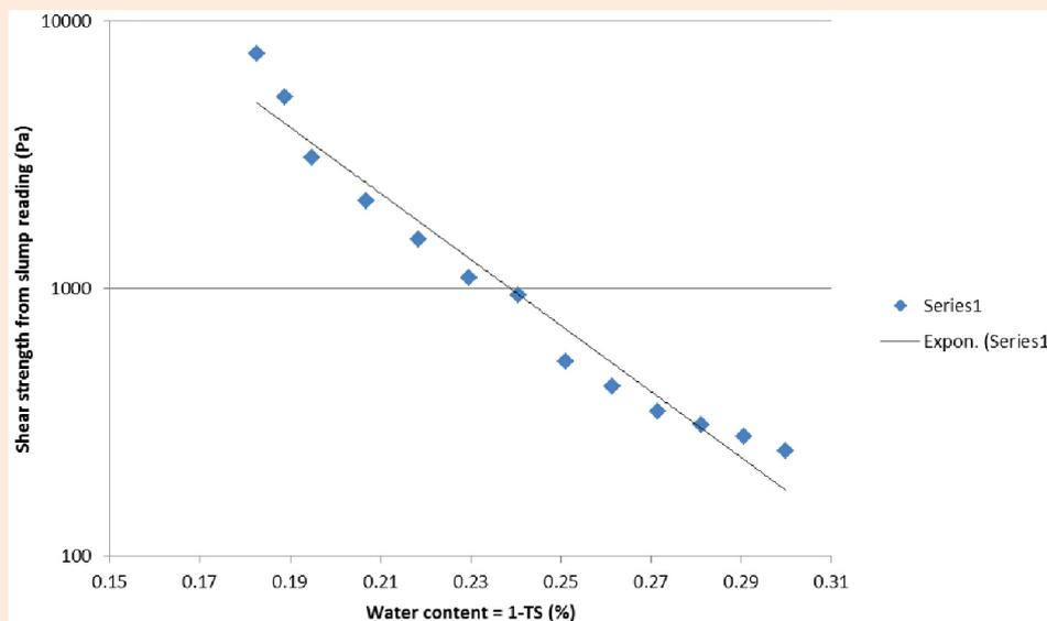
Figure 1: shear strength from slump reading versus water content
