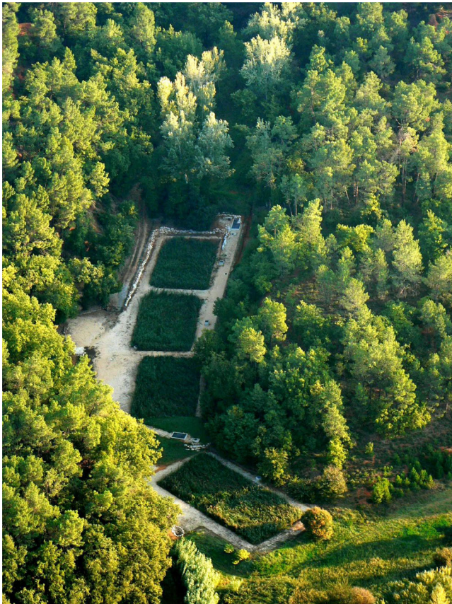
Figure 5.7 Aerial view of the Roussillon French VF wetland. Photo courtesy of Vincent Leboeuf, SYNTEA group.
